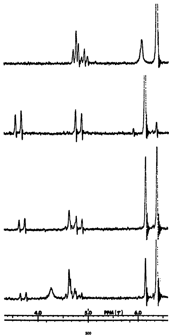
Figure 1.—Main features of typical nmr spectra for the reaction of erythro amido esters with thionyl chloride. Top: erythro - N -benzoyl- \beta -phenylserine methyl ester ( erythro 2) in \text{CDCl}_3 (broad resonance at ca. 235 cps in OH). Second: one minute after addition of thionyl chloride, trans -4-carbomethoxy-2,5-diphenyl-2-oxazoline hydrochloride ( trans 8). Third: one hour; about 50% conversion of trans 8 into erythro - N -benzoyl- \beta -chloro- \beta -phenylalanine methyl ester ( erythro 12). Bottom: conversion into erythro 12 is 75%; broad "mobile" peak at ca. 345 cps moves upfield throughout reaction.
